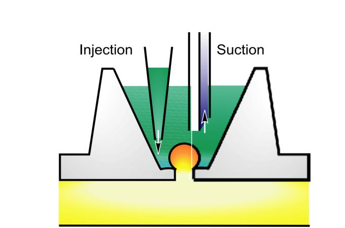
Methods used in the conventional patch-clamp technique and PatchXpress 7000A. A; Principle diagrams of measurement in the conventional and automated patch-clamping. B; Schematic diagrams of exchange of extra-cellar solution in the conventional and automated patch-clamping.
